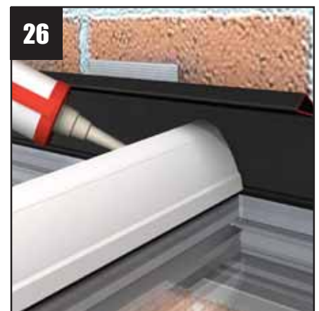
26 Seal along the back edge of the glazing around the top capping where they meet the rain baffle.
