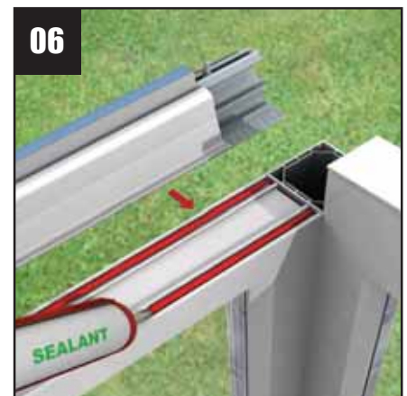
Take the eaves beam and make sure the head of the front frame is siliconed.
