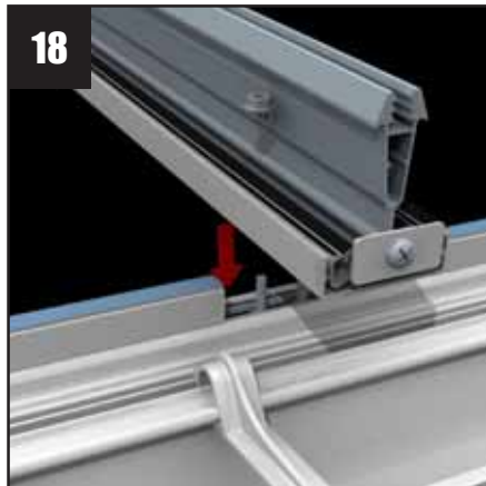
18 Attach all the glazing bars using the location plan provided to check each bars final position with its corresponding label.
