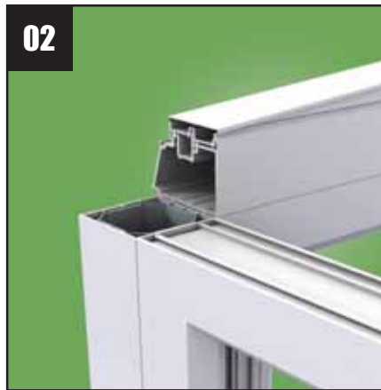
Each furring is 45mm longer than the internal frame projection. When cutting the furring, always do this at the back (rear) and ensure that all elements are in aligned.
