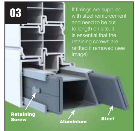
Unpack and slide in the aluminium box section (if ordered) and, the two pieces of steel re-inforcing (if ordered). If only one section of stage 1 re-inforcing is supplied it usually signifies that this should be used above doors in the side elevation.
