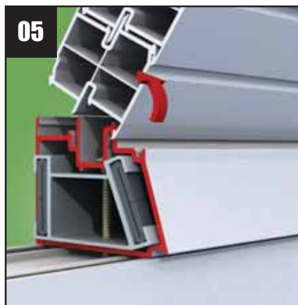
Use the 4.8 diameter x 70mm fixing supplied at 450mm centres and within 200mm of the corners. Now, reassemble the furring by clipping in the bottom edge of the furring top section and roll into place.
